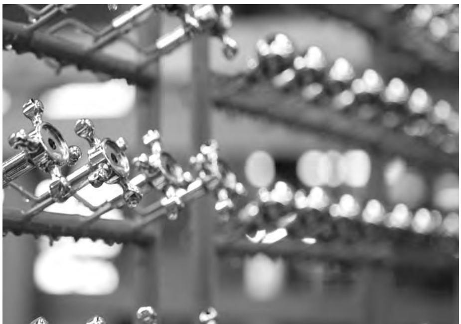
CROSSTOP HANDLE BOSSES ARE RACKED AND PLATED IN-HOUSE
