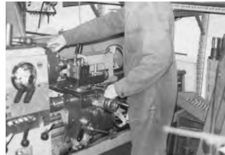
SCREWCUTTING WASHER PLATES FOR A CUSTOMER
