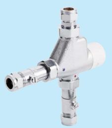
MT503CP-22 - A 15mm blending valve with 22mm Compression inlets. Suitable for high pressure bath fills, the MT503 CP-22 has 22mm inlets and 15mm outlet. Check valves and serviceable filters are supplied as standard.
